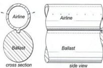
0.75 HP Oil-less Rocker Piston Compressors, 7.3 CFM Air Supply 150' of 1/2" ID Self Weighted Bubble Tubing®; with Two Check Valve Kits
