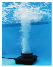
Membrane air diffuser assemblies feature round rubber membrane with thousands of holes which produce small air bubbles when supplied with air from an on shore compressor. These bubble rise to the surface and create circulation that helps destratify and aerate the water body.
