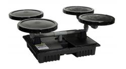
Membrane air diffuser assemblies feature round rubber membrane with thousands of holes which produce small air bubbles when supplied with air from an on shore compressor. These bubble rise to the surface and create circulation that helps destratify and aerate the water body.
